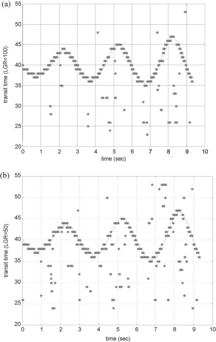
Fig. 4. An example of the effect of increasing amounts of global component on transit time estimation for the flow regime of oscillating with increasing amplitude transit time; estimated transit time (thick, light lines) overlapped with the actual transit time (thin, dark lines) for LGR = 100, 50, 25 and 15.
