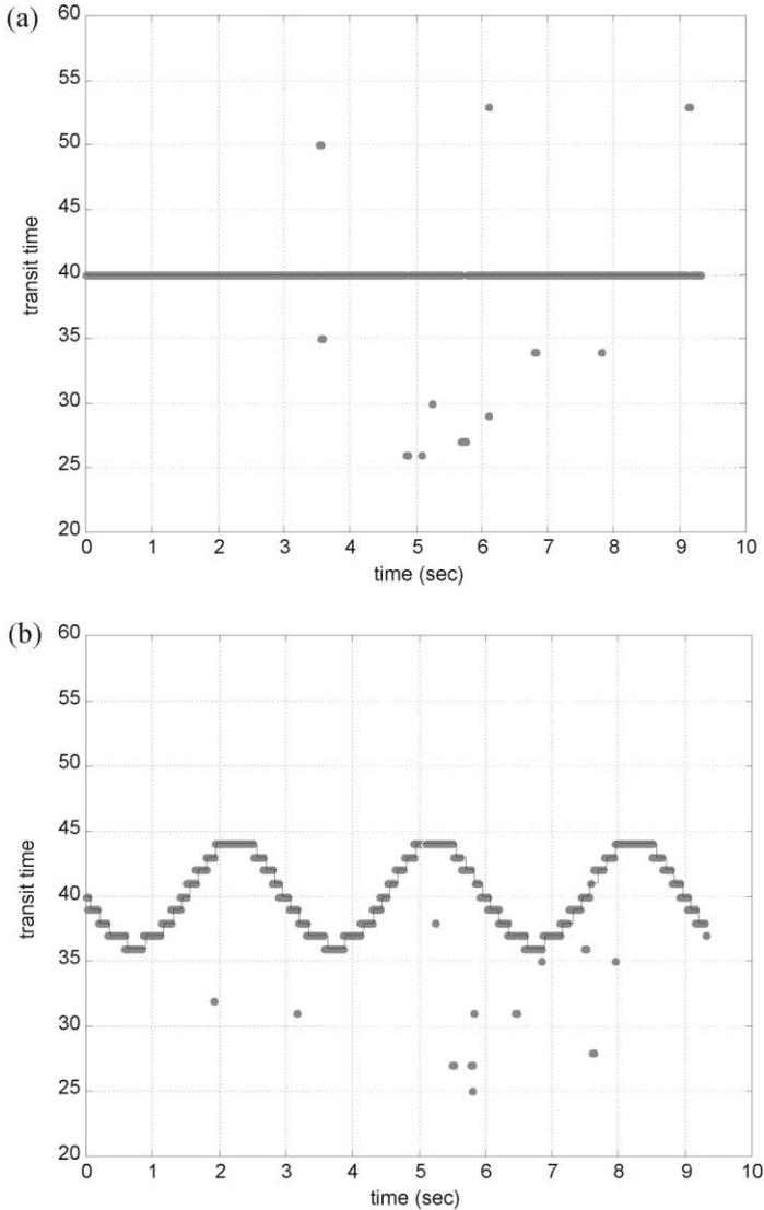
Fig. 3. Representative examples of transit time estimation for the flow regimes of constant (a), oscillating with constant amplitude (b), oscillating with increasing amplitude (c), and decreasing whilst oscillating with constant amplitude (d) transit time; estimated transit time (thick, light lines) overlapped with the actual transit time (thin, dark lines).
