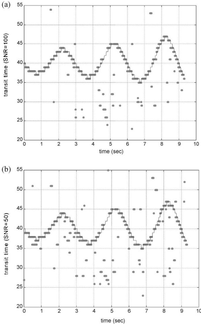
Fig. 5. An example of the effect of increasing amounts of uncorrelated white noise on transit time estimation for the flow regime of oscillating with increasing amplitude transit time; estimated transit time (thick, light lines) overlapped with the actual transit time (thin, dark lines) for SNR = 100, 50, 25 and 15.
