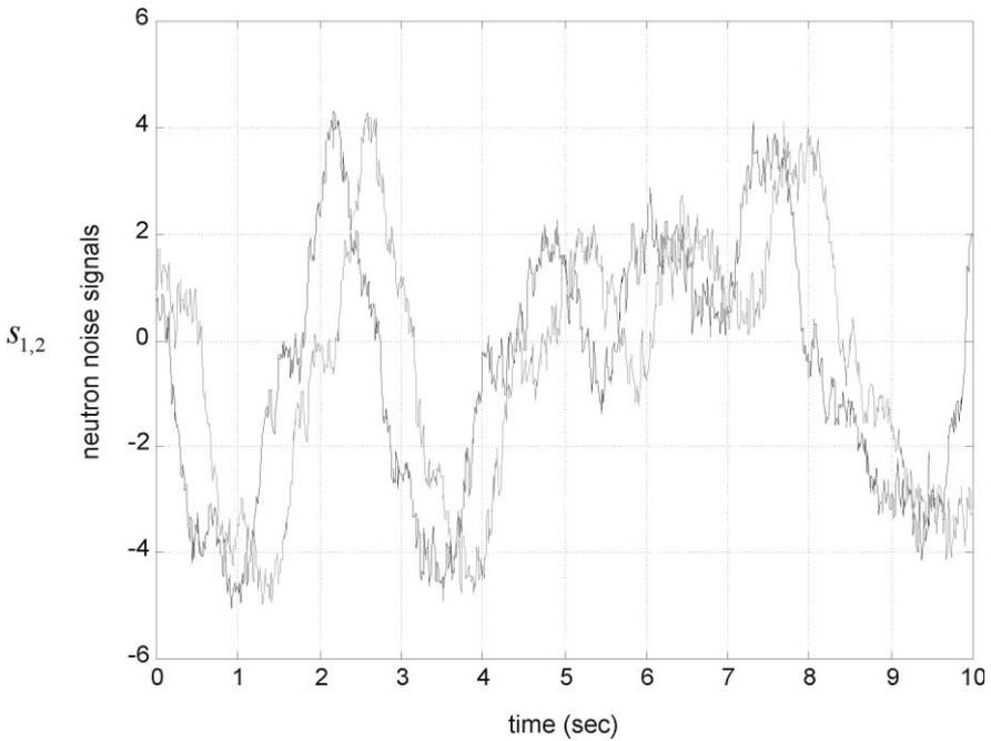
Fig. 1. Neutron noise signals  $s_1$  and  $s_2$  collected at  $D_1$  (dark line) and  $D_2$  (light line), respectively, for the flow regime of oscillating with increasing amplitude transit time.
