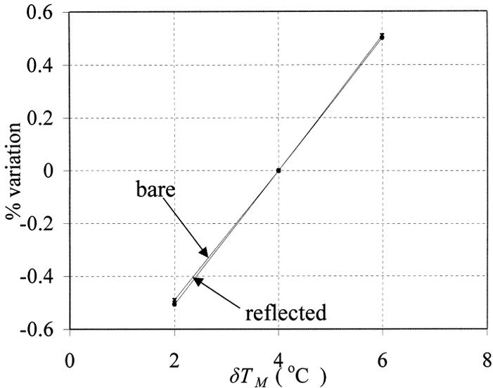
Fig. 4. Percentage variation of MTC as a function of moderator temperature change  $\delta T_M$ .; >
