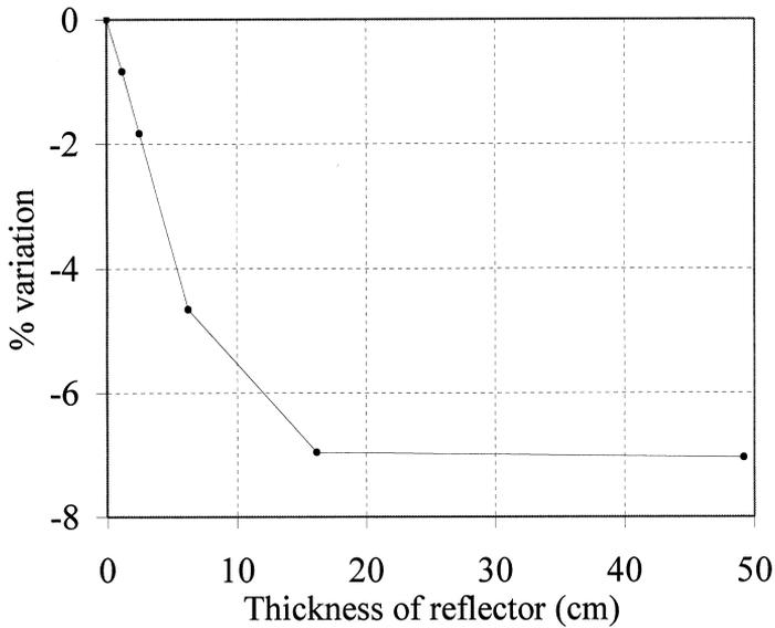
Fig. 3. Percentage variation of MTC as a function of thickness of reflector for a small core ( $H=100$  cm,  $W=100$  cm).; >
