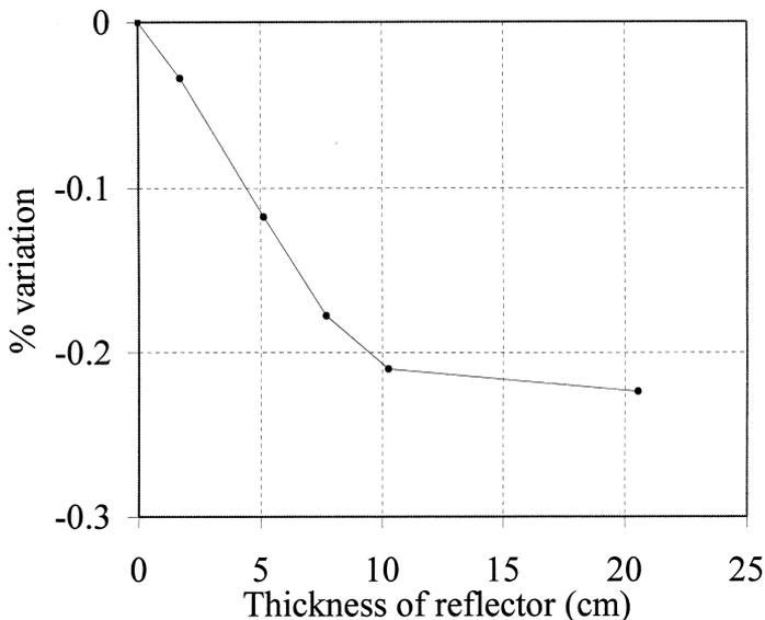
Fig. 2. Percentage variation of MTC as a function of thickness of reflector for a large core ( $H = 370$  cm,  $W = 340$  cm).;: >
